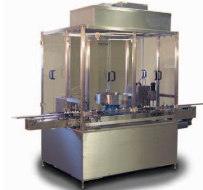
Automatic Liquid Fill and Finish machine, IntelliTech, Inc.
